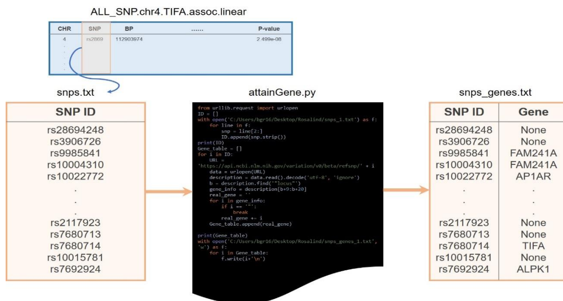
Figure 1. Python Programming Scheme of attaining gene name from the dbSNP. When the text file containing SNPs' ID, which is extracted from the association file were input, attainGene.py would be executed and access to the https://api.ncbi.nlm.nih.gov/variation/v0/beta/refsnp/ “SNPid” according to each SNPid. After the execution, each SNPs would obtain the information whether they are in the gene or not and saved into snps_genes.txt file.
